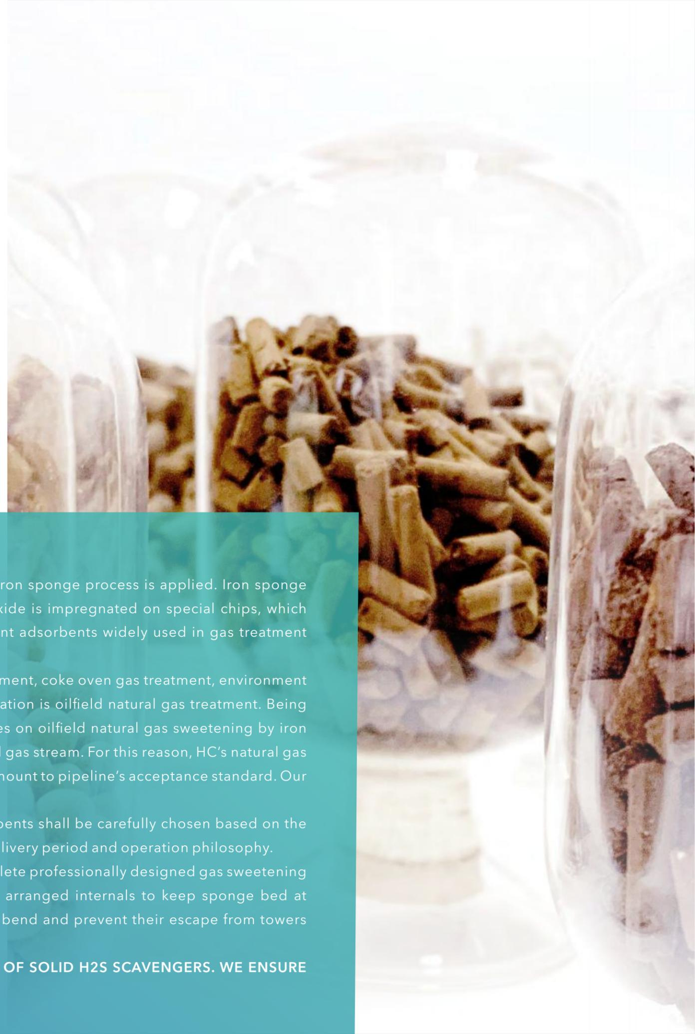
Iron sponge (Solid H<sub>2</sub>S Scavenger) is a special granular solid which is widely used in gas sweetening where iron sponge process is applied. Iron sponge process employs iron oxide which reacts with hydrogen sulfide (H<sub>2</sub>S) forming iron sulfide and water. Iron oxide is impregnated on special chips, which contain other chemical additives to increase efficiency of solid bed scavengers. Iron sponge is a very efficient adsorbent widely used in gas treatment processes.
